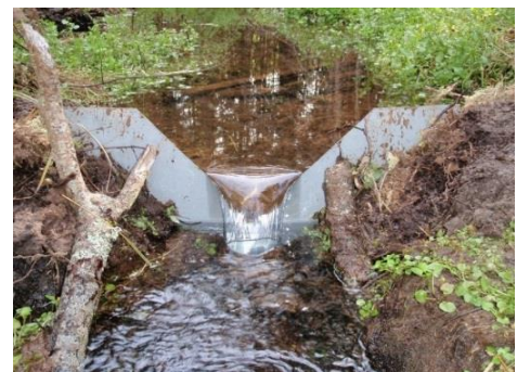
V-notch from weir to measure streamflow.
